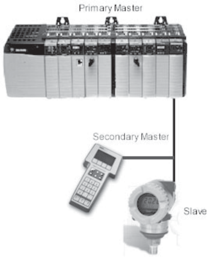
Figure 7.3 (Primary, Secondary and Slave connection)
