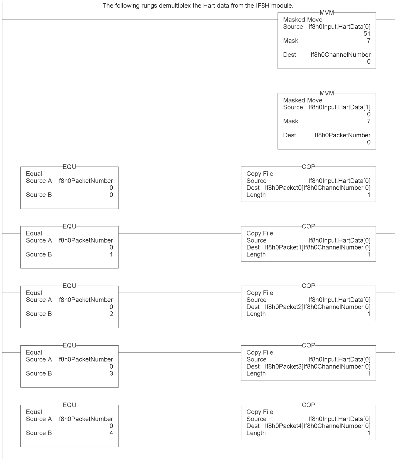
Figure 8.2 (IF8H Demultiplexing Ladder)
