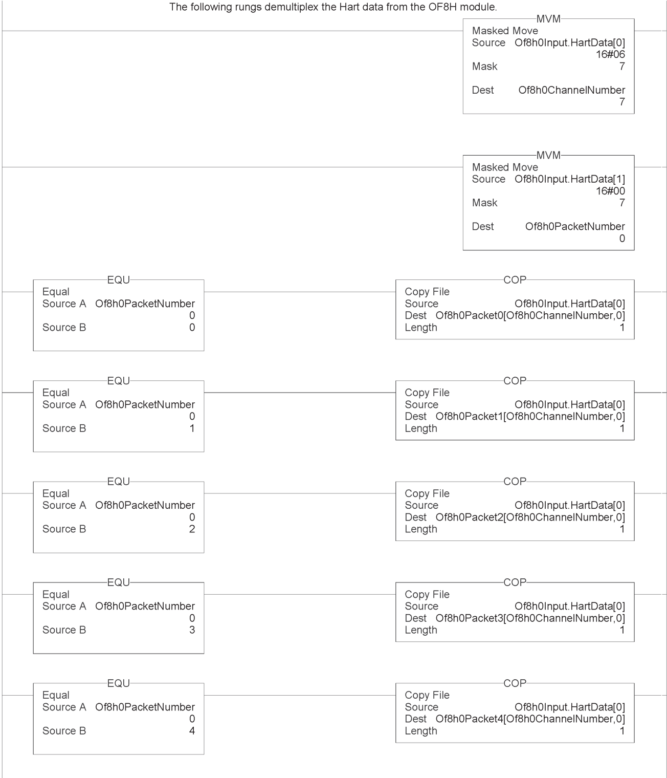
Figure 8.3 (OF8H Demultiplexing Ladder)
